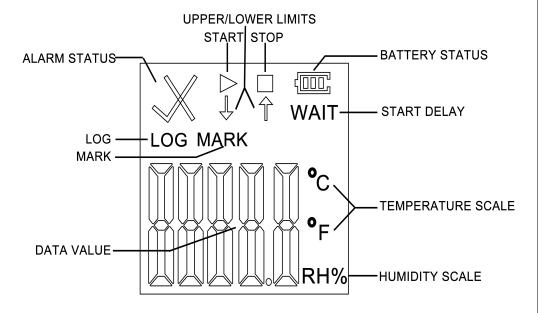
During normal use, press " $\blacktriangleright$ " to switch the screen display interface. The data logger display interfaces include: real-time temperature display  $\rightarrow$  real-time humidity display  $\rightarrow$  LOG interface  $\rightarrow$  MARK interface  $\rightarrow$  temperature upper limit display  $\rightarrow$  temperature lower limit display  $\rightarrow$  humidity upper limit display  $\rightarrow$  humidity lower limit display.
